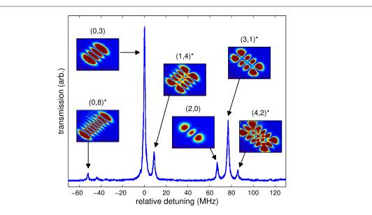
**Figure 3.** Transverse cavity modes. The solid curve shows a number of cavity transmission resonances (without atoms), and insets show the corresponding spatial profiles as imaged onto a camera. The  $45^{\circ}$  tilt of the patterns reflects the orientation of the cavity plane ( $\searrow$ ). The modes are labelled according to transverse indices (m, n), with asterisks denoting a longitudinal index q which is one less than that of the (0, 3) mode which is taken as reference.
